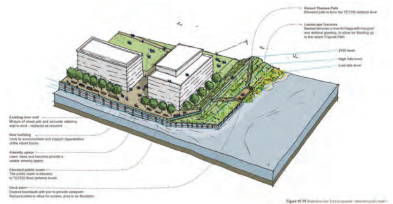
Setting back the defence line to create better public access to the estuary Source: Environment Agency
