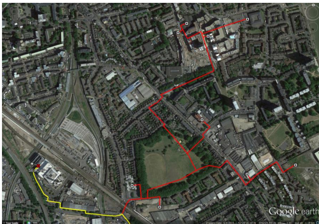
Figure 8-1: Alternative route minimising installation in Evelyn Street
