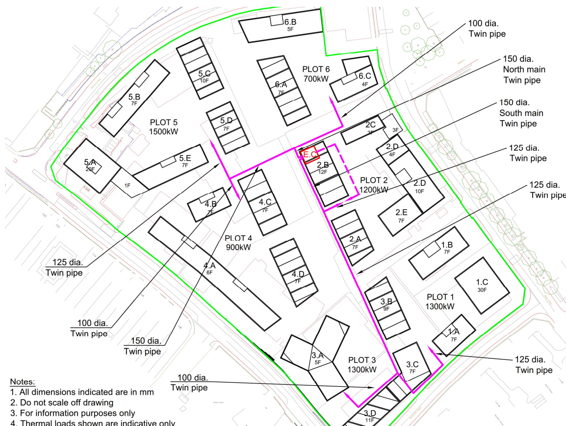
Figure 4-2: The Wharves Deptford proposed EC location (red box) and DH pipework route
