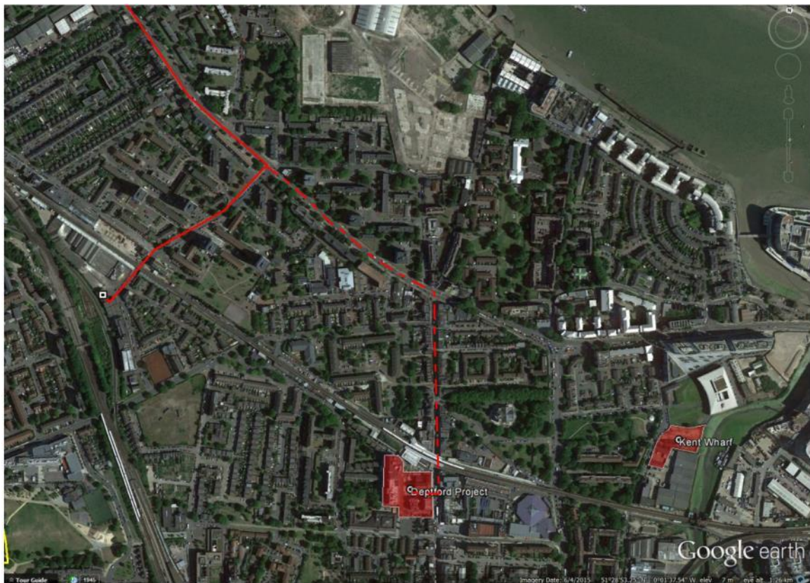
Figure 5-5: Network extension to the Deptford Project
