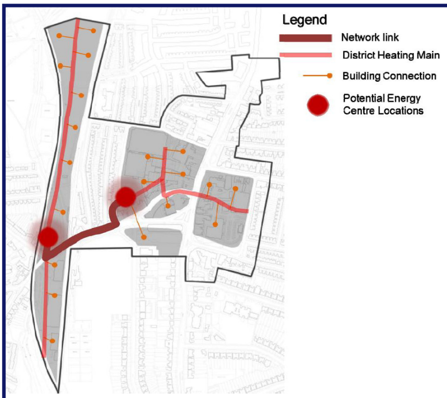
Figure 5.3: Potential locations for energy centres
