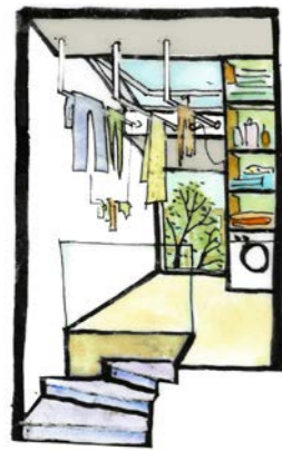
Fig. 45: Skylight over a laundry landing
