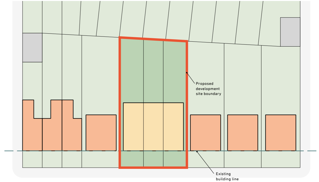
Fig. 104: By removing a single dwelling which fails to make optimum use of its site and replacing it with new homes can deliver new family homes while repairing the streetscape.
